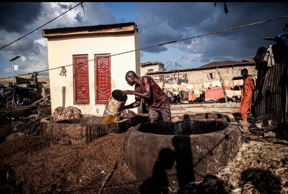
Tan gent: A Majama worker changes the water in a tanning pit, readying it for the next processing run.
