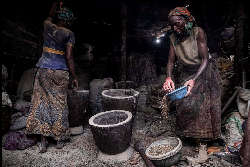
Sift shift: Aliyu Garba's sisters pound acacia seeds into бага ruwa powder in the tannery's backyard. This powder is essential in the softening process of the hide.
